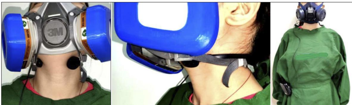
Figure 2. Laryngophone receivers positioned at the level of the hyoid and speaker attached to the protective gown.
