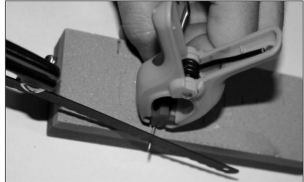
Figure 2. Cutting the distal tip of the alligator forceps using a hacksaw
