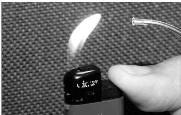
Figure 7. Flanging the tube
