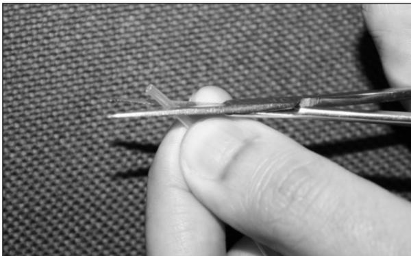
Figure 6. Cutting the polyethylene tube
