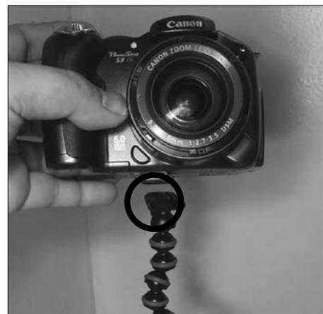
Figure 7b. Camera with attached quick release plate (circle)
