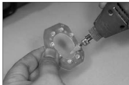
**Figure 4.** A 33mm hole cut was into the circuit board
