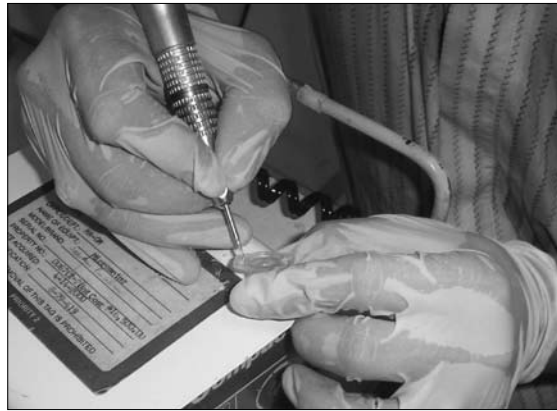
Figure 5. Holes for string attachment created on both sides of the neck plate of the barrel using a hand drill.
