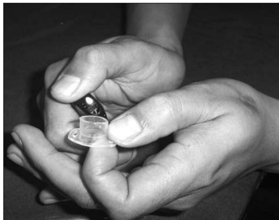
Figure 6. Sharp edges of the cut syringe smoothed with a flame.
